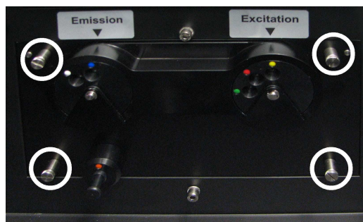
Figure 28: Filter change/Filter installation: Loosen the 4 screws
