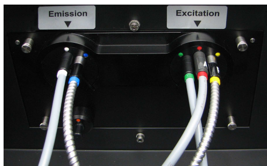
Figure 27: Filter change/Filter installation: First remove the optic (valid for all readers)
