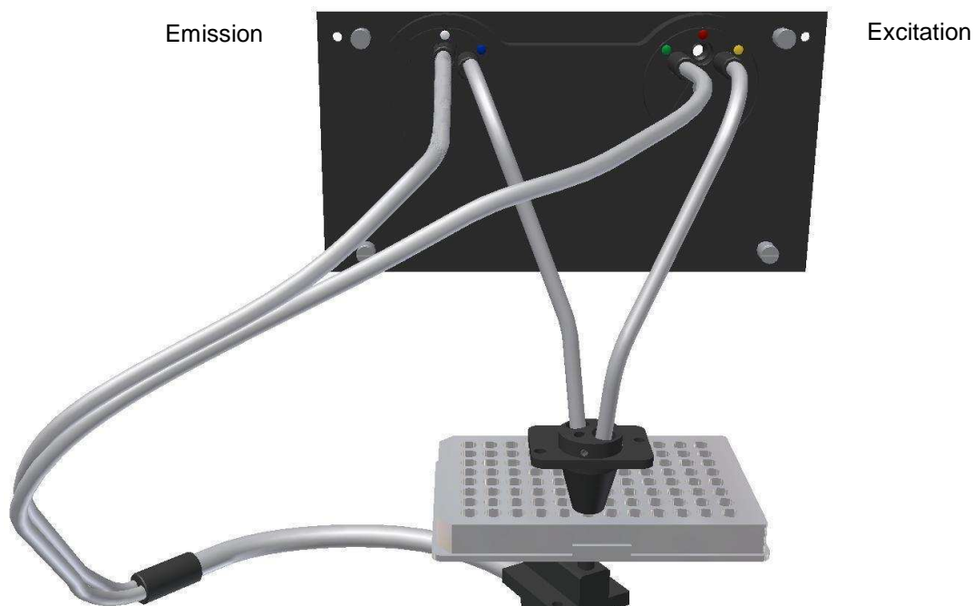
Figure 22: Principle drawing of bottom reading of a 96 well plate
