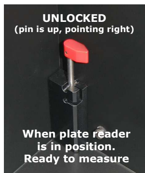
Figure 2: Left: transport pin in locked position (pin is down). Middle: transport pin in unlocked position (pin is up). Right: the groove where the transport pin can lock the plate carrier
